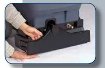
Floating vacuum shoe follows the contour of the carpet for superior recovery.
