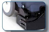
Brush setting easily adjusts to eight cleaning positions for maximum performance and a storage position increases brush life.
